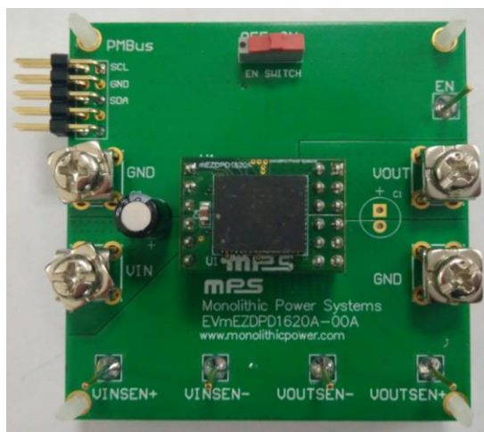
Figure 2: EVmEZDPD1620A-00A Evaluation Board
