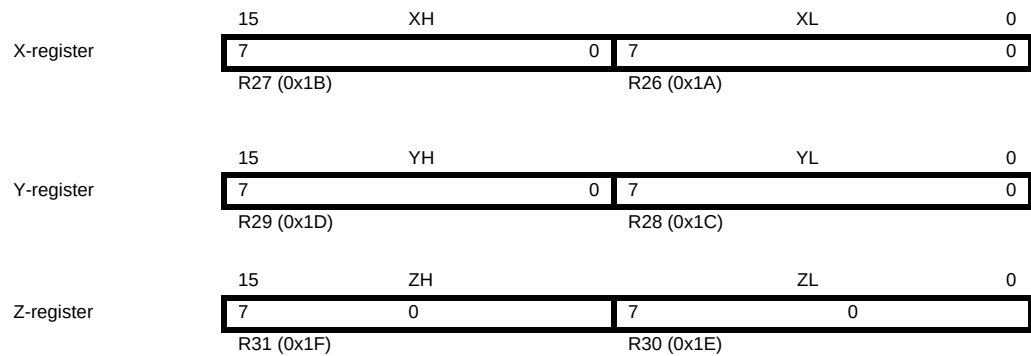
Figure 3-3. The X-, Y-, and Z-registers
