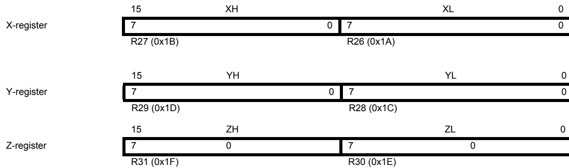
Figure 4-3. The X-, Y-, and Z-registers
