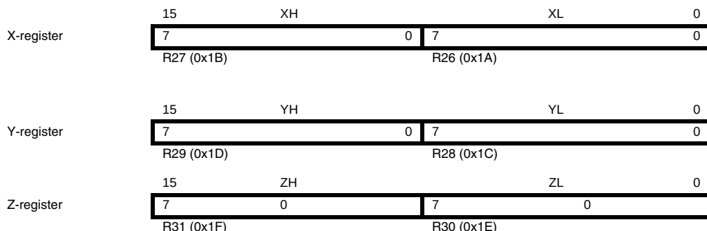
Figure 4-3. The X-, Y-, and Z-registers
