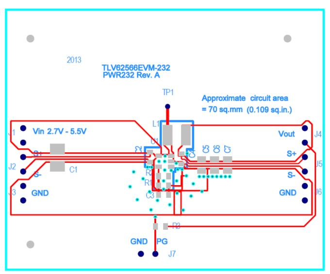
Figure 2. Assembly Layer
