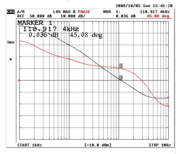
Figure 1. Bode Plot with  $V_{IN}$  = 3.6 V,  $V_{OUT}$  = 1.8 V,  $I_{OUT}$  = 1 A
