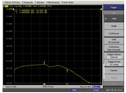
Figure 5-9. Coupling between left and right antennas.
