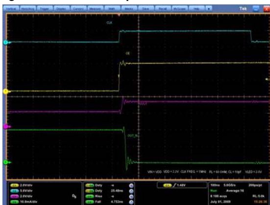
Figure 16: Turn ON output current characteristics (1)
