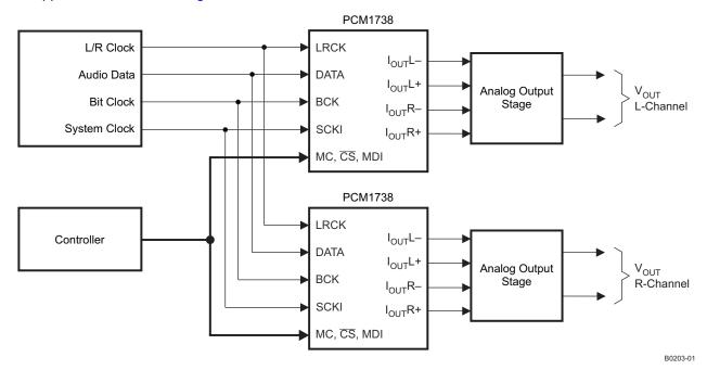
Figure 47. Connection Diagram for Monaural-Mode Interface
