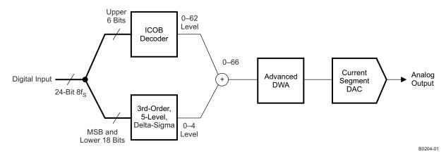
Figure 48. Architecture of Advanced Segment DAC
