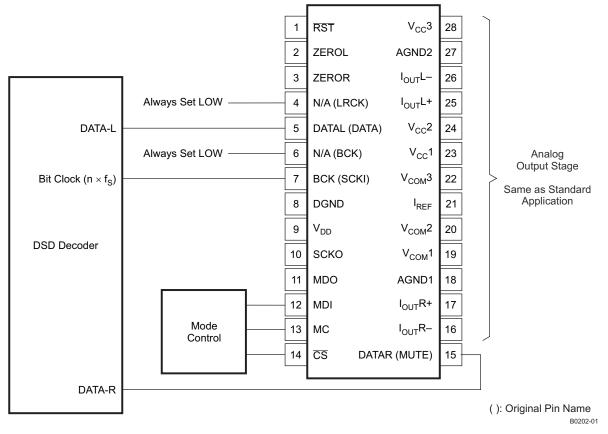
Figure 44. Connection Diagram for DSD Format Interface
