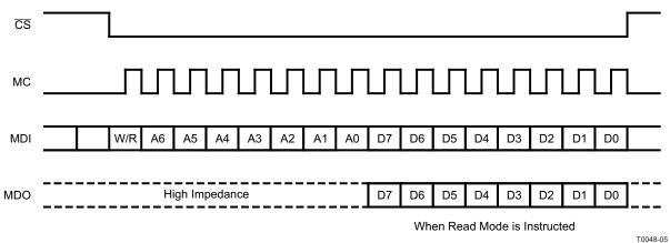
NOTE: B15 is used for the selection of write or read. Setting W/R = 0 indicates a write, while W/R = 1 indicates a read. B14-B8 are used for the register address. B7–B0 are used for frgister data.
