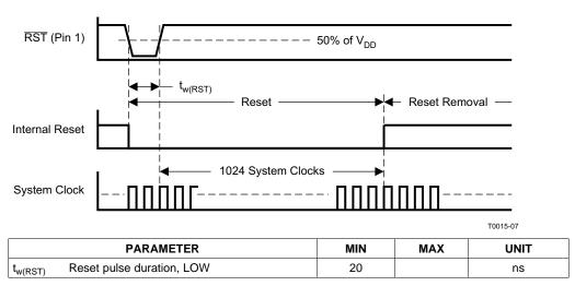
Figure 34. External Reset Timing
