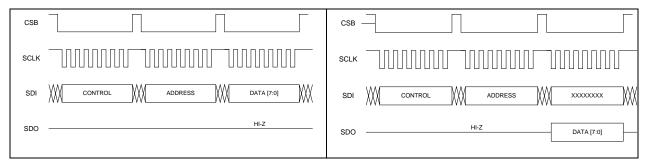
Figure 1: SPI Write Transaction
