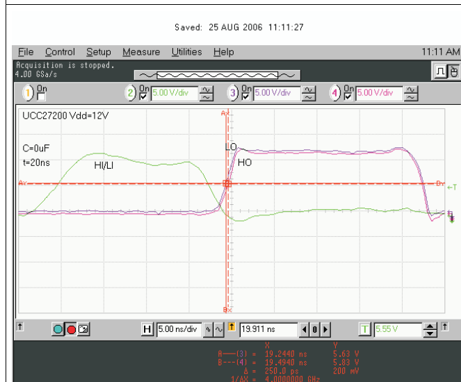
Figure 27. 20-ns Input Pulse Delay Matching
