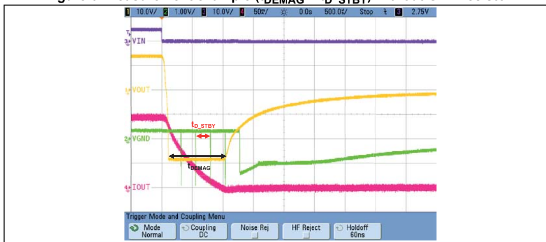
Figure 6. Measurement example ( t_{\text{DEMAG}} > t_{\text{D\_STBY}} ) without GND resistor
