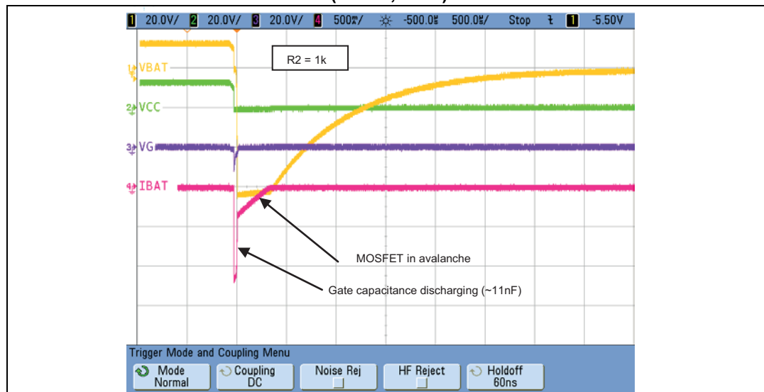
Figure 12. MOSFET solution in V_{CC} – experiment VND7020AJ, ISO pulse 1 (-100 V, 90 \Omega )
