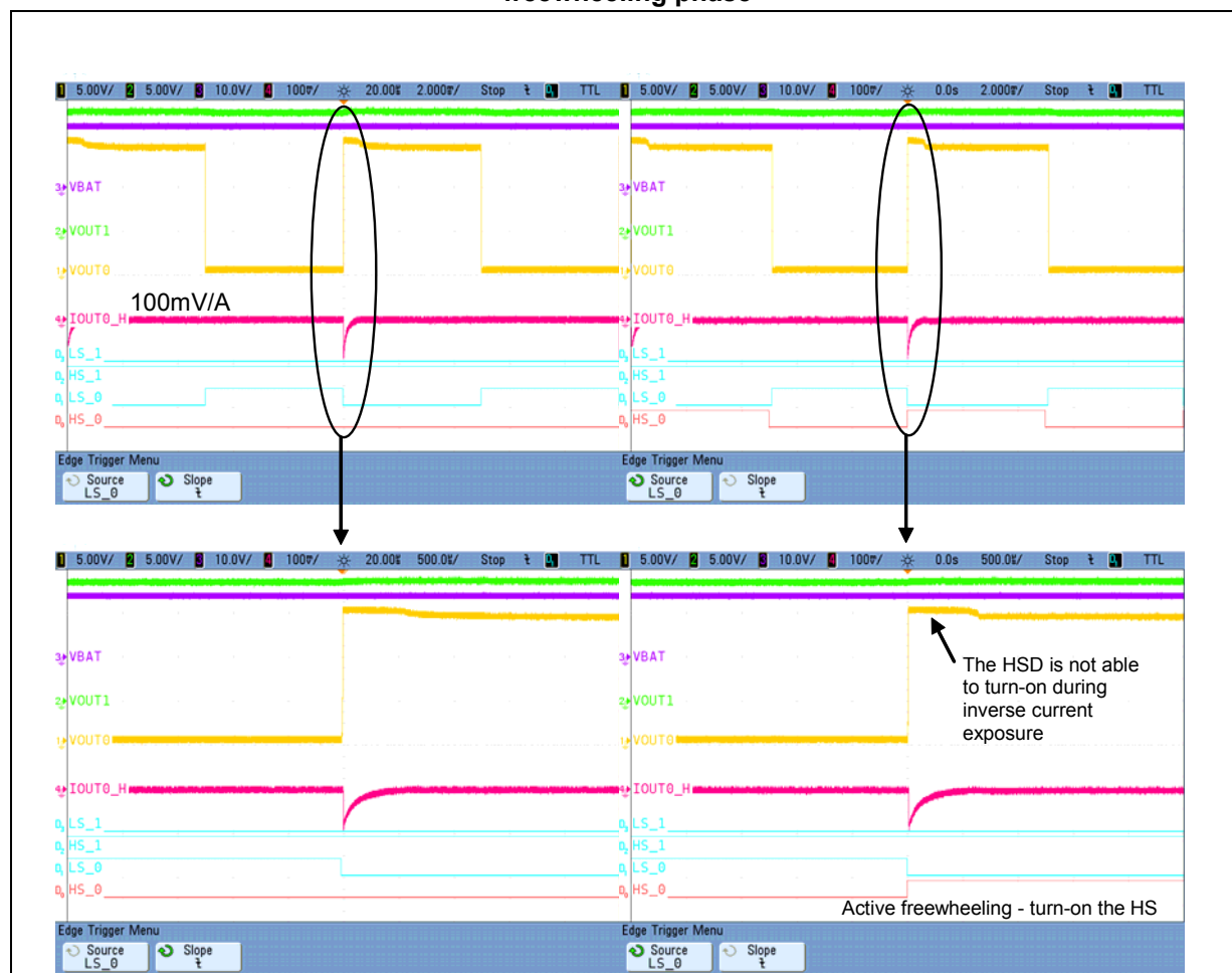
Figure 164. H-Bridge formed by one VND7140AJ and two OMNIFETs II showing the high-side freewheeling phase
