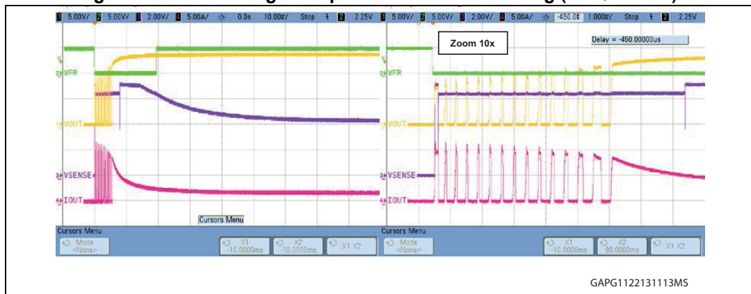
Figure 31. FR handling example - bulb inrush blanking (VNQ7140AJ)
