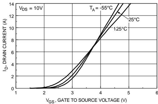
Figure 5. Transfer Characteristics.
