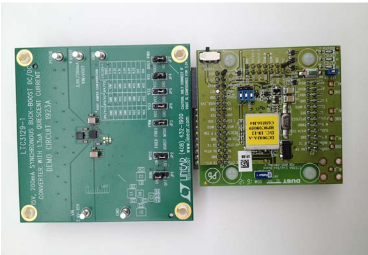
Figure 5. DC1923A Connected to DC9003A Dust Mote (Top View)
