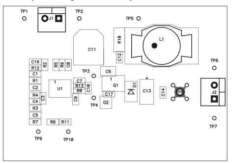
Figure 8. Top Side Component Assembly
