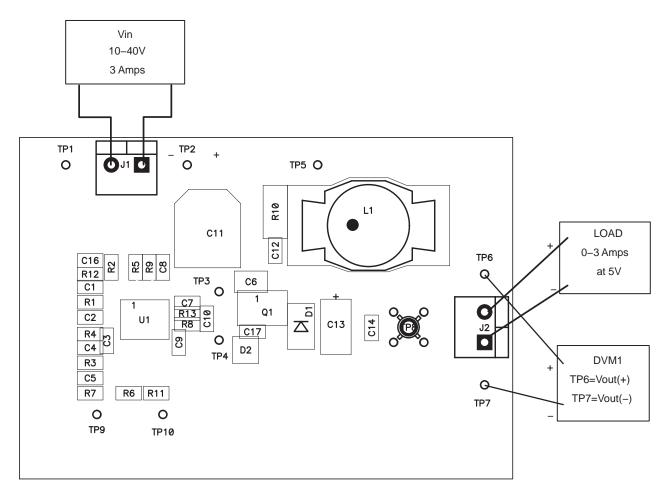
Figure 2. Test Setup
