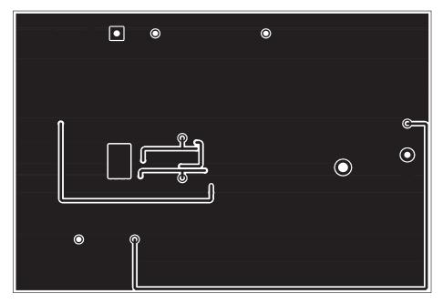
Figure 10. Bottom Layer Copper
