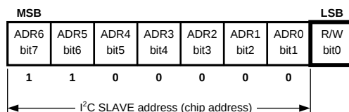
Figure 21. I 2 C Chip Address (see NOTE above)
