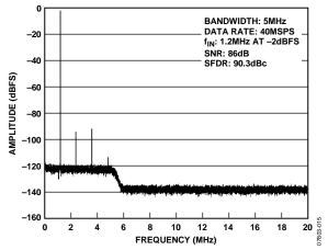
Figure 5. Single-Tone FFT with  $f_{\rm IN}$  = 1.2 MHz and BW = 5 MHz
