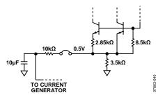
Figure 40. Internal Reference Configuration
