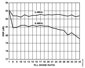
Figure 20. Single-Tone SNR vs. PLL Divide Ratio
