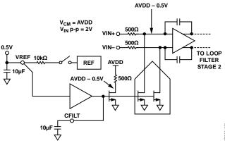
Figure 39. Voltage Reference Loop
