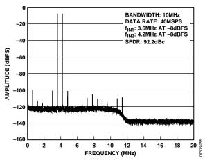
Figure 12. Two-Tone FFT with  $f_{\text{IN1}} = 3.6$  MHz and  $f_{\text{IN2}} = 4.2$  MHz
