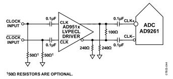
Figure 44. Differential LVPECL Sample Clock
