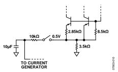
Figure 28. Equivalent VREF Circuit
