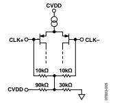
Figure 23. Equivalent Clock Input Circuit
