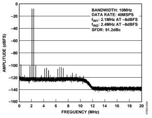
Figure 11. Two-Tone FFT with  $f_{\rm IN1}$  = 2.1 MHz and  $f_{\rm IN2}$  = 2.4 MHz
