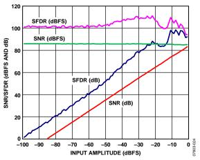
Figure 14. Single-Tone SNR and SFDR vs. Input Amplitude with  $f_{IN} = 2.4$  MHz
