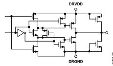
Figure 27. Equivalent Digital Output Circuit
