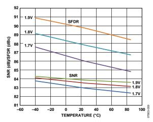
Figure 18. SFDR/SNR vs. Temperature with  $f_{IN} = 2.4 \text{ MHz}$
