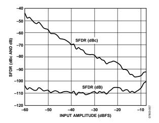
Figure 15. Two-Tone SFDR/IMD3 vs. Input Amplitude with  $f_{\rm IN1}=2.1$  MHz and  $f_{\rm IN2}=2.4$  MHz
