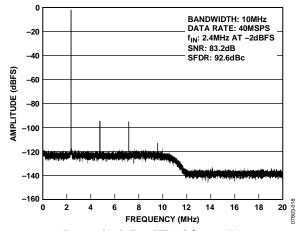
Figure 8. Single-Tone FFT with  $f_{\rm IN}$  = 2.4 MHz
