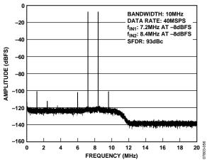
Figure 13. Two-Tone FFT with  $f_{\text{IN1}} = 7.2$  MHz and  $f_{\text{IN2}} = 8.4$  MHz
