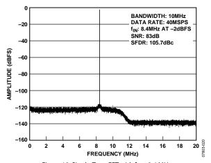
Figure 10. Single-Tone FFT with  $f_{\rm IN} = 8.4~\rm MHz$
