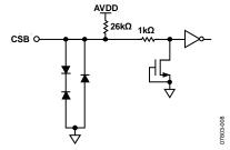
Figure 26. Equivalent CSB Input Circuit
