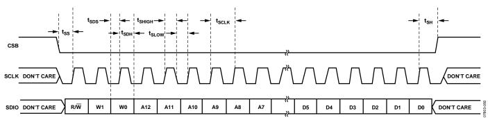
Figure 50. Serial Port Interface Timing Diagram
