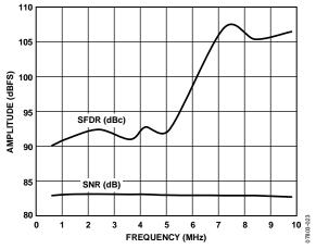
Figure 17. SNR/SFDR vs. Input Frequency
