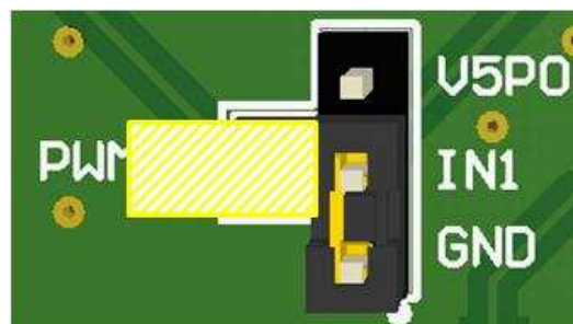
Figure 6. IN1 Floating, can be Controlled Externally
