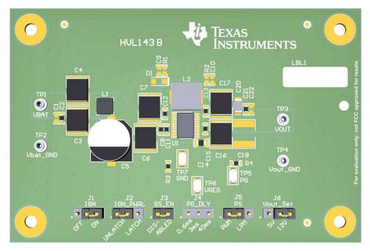
Figure 6. Component Placement—Top
