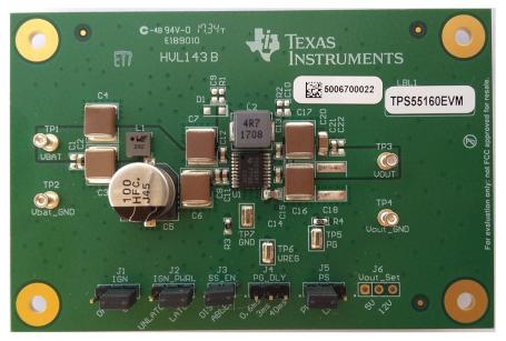
Figure 1. TPS55160Q1-EVM With Jumper Settings
