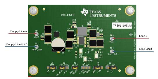
Figure 16. TPS55165Q1-EVM Showing Supply and Load Connections
