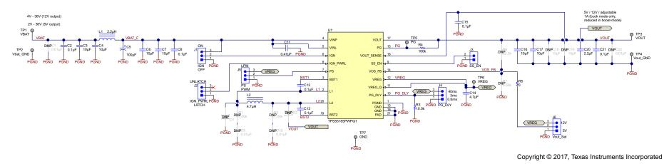
Figure 4. TPS55160Q1-EVM Schematic Diagram—Assembly Option
