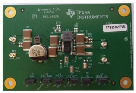
Figure 2. TPS55165Q1-EVM With Jumper Settings
