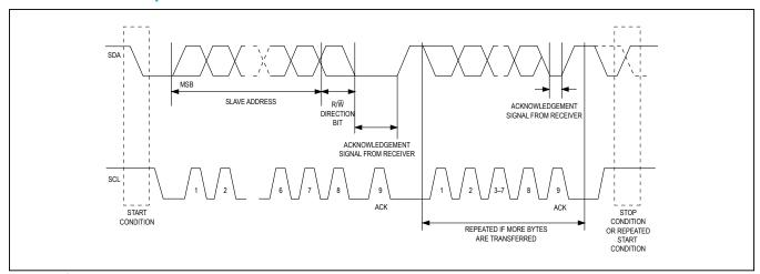
Figure 3. I2C Data Transfer Protocol
