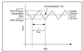
Figure 2. Output Frequency vs. Dither Rate
