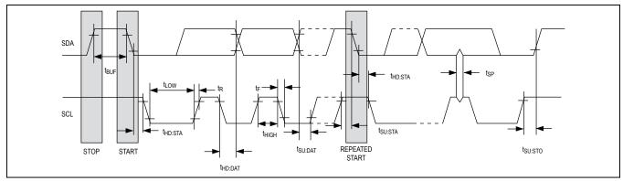
Figure 5. I2C AC Characteristics
