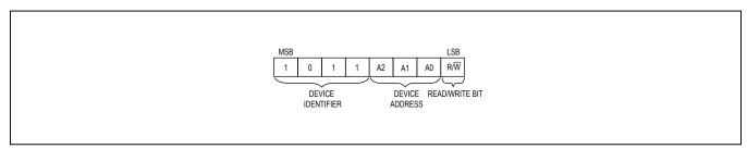
Figure 4. Slave Address Byte
