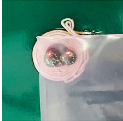
Figure 10. DC2687A (2 in bag) on DC2261A coil
