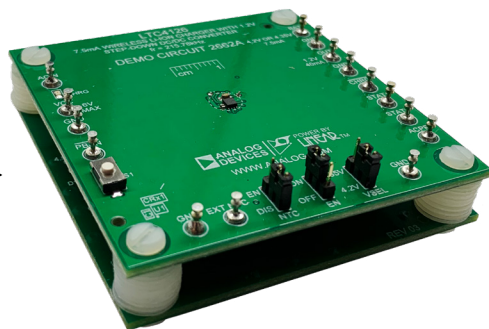
Figure 7. DC2662A mounted on top of DC2661A
