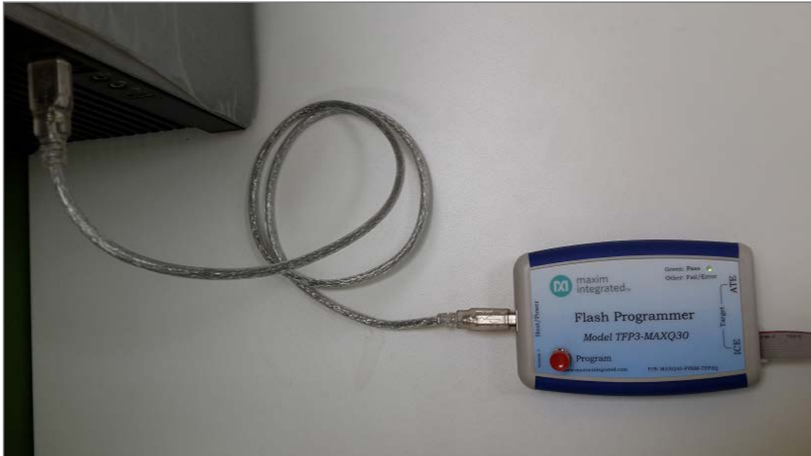
Figure 2: TFP3 Connection to Host
