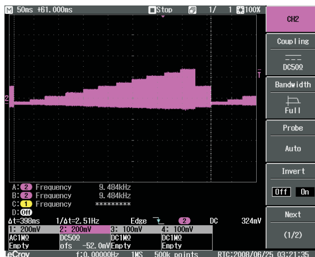
Figure 7. TSW7001 Ramp Output
