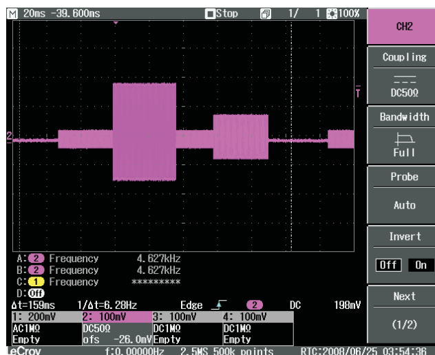
Figure 9. Output of TSW7001 With Arbitrary Gain Profile
