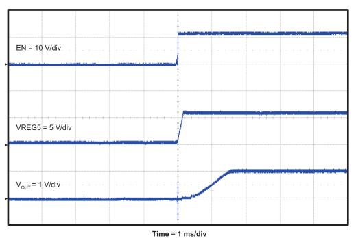
Figure 9. TPS54526EVM-608 Start Up Relative to Enable
