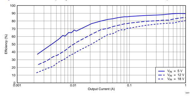
Figure 2 shows the efficiency at light loads for the TPS54526EVM-608 at an ambient temperature of 25°C.
