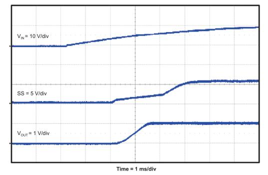
The TPS54526EVM-608 start up waveform relative to  $V_{IN}$  is shown in Figure 8.
