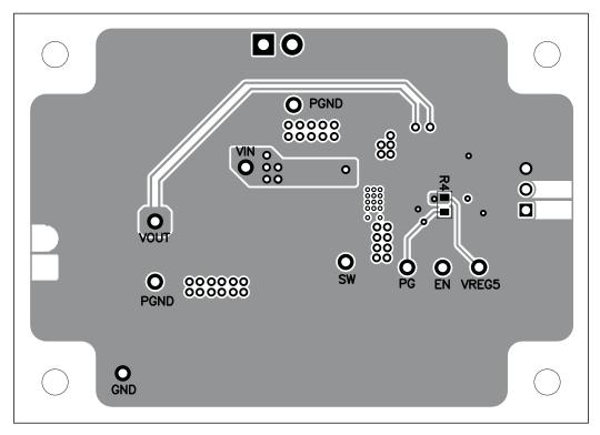
Figure 15. Bottom Assembly as Seen from Back Side
