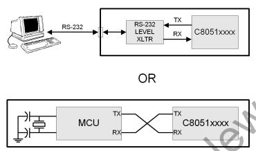
Figure 25.3. UART Interconnect Diagram
