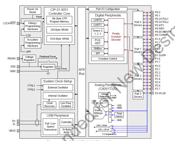
Figure 1.3. C8051T320/2 Block Diagram
