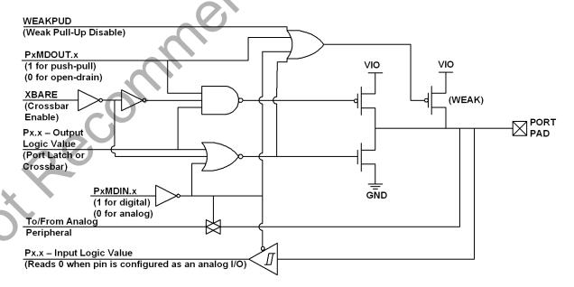
Figure 22.2. Port I/O Cell Block Diagram
