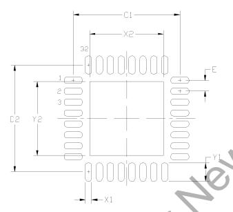
Figure 5.2. QFN-32 Recommended PCB Land Pattern
