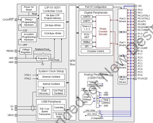
Figure 1.1. C8051T620/1 Block Diagram
