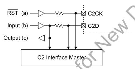
Figure 30.1. Typical C2 Pin Sharing
