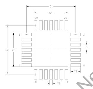
Figure 6.2. QFN-28 Recommended PCB Land Pattern
