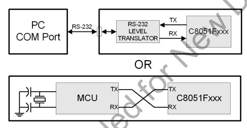
Figure 26.5. Typical UART Interconnect Diagram
