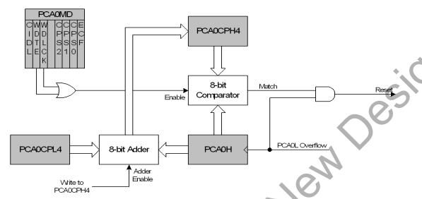
Figure 29.11. PCA Module 2 with Watchdog Timer Enabled
