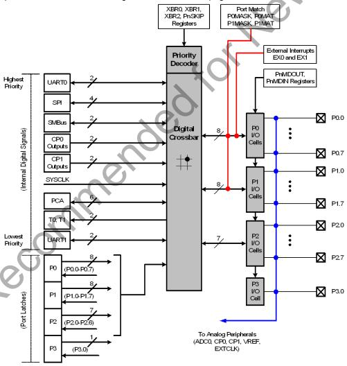
Figure 22.1. Port I/O Functional Block Diagram
