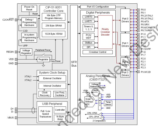
Figure 1.4. C8051T321/3 Block Diagram
