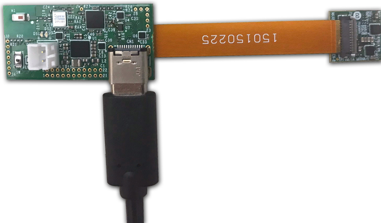
Figure 9. Hardware Setup (MAX86140 EVSYS Micro-PCB)
