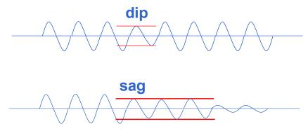
Figure 5-22: Sag and Dip Conditions
