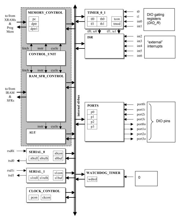
Figure 6-2: 80515 MPU Block Diagram
