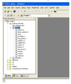
The Project Workspace screen on the left side of the window shows the main components of the source (Startup and main, Metering, CE, IO, Utilities, Command Line Interface) in folders. Folders can be opened by clicking on the plus sign next to them. Opening the folders will display the source files associated with them. Opening the source files will display the header files used by them.
