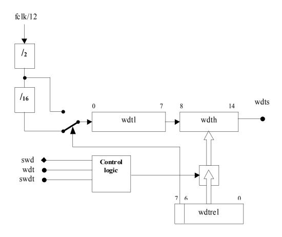
Figure 6-3: Watchdog Block Diagram
