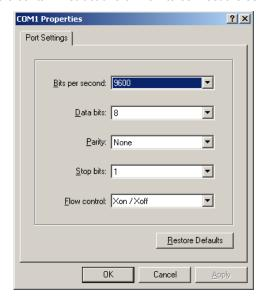
Figure 3-1: Port Speed and Handshake Setup (left) and Port Configuration Setup (right)
