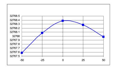
Figure 5-24: Crystal Frequency over Temperature
