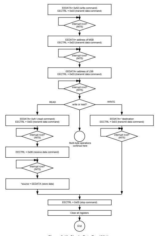
Figure 5-19: Single-Byte Read/Write
