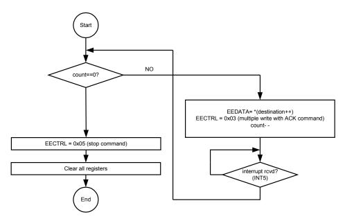
Figure 5-21: Multi-Byte Write
