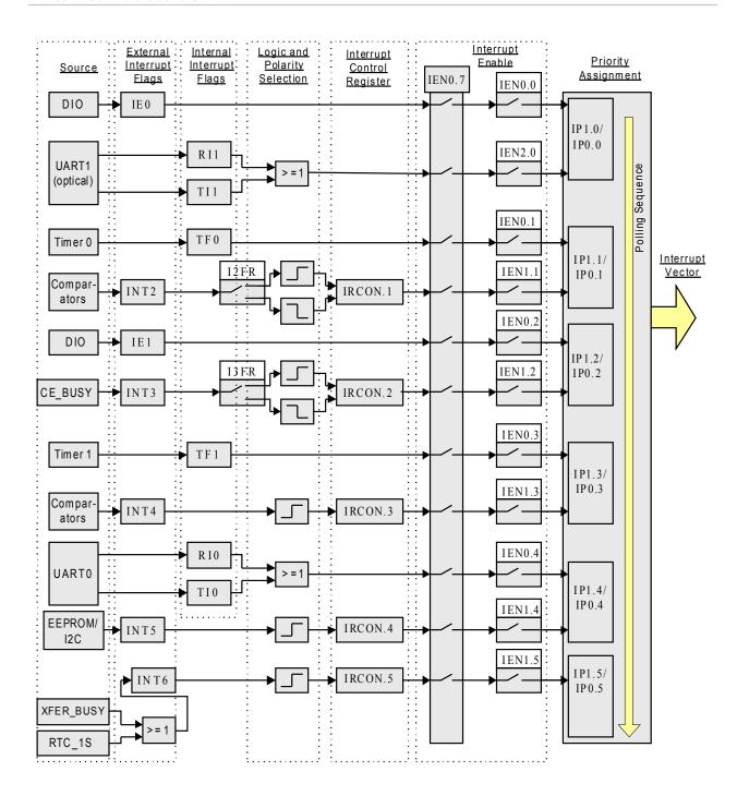
Figure 6-4: Interrupt Sources Diagram
