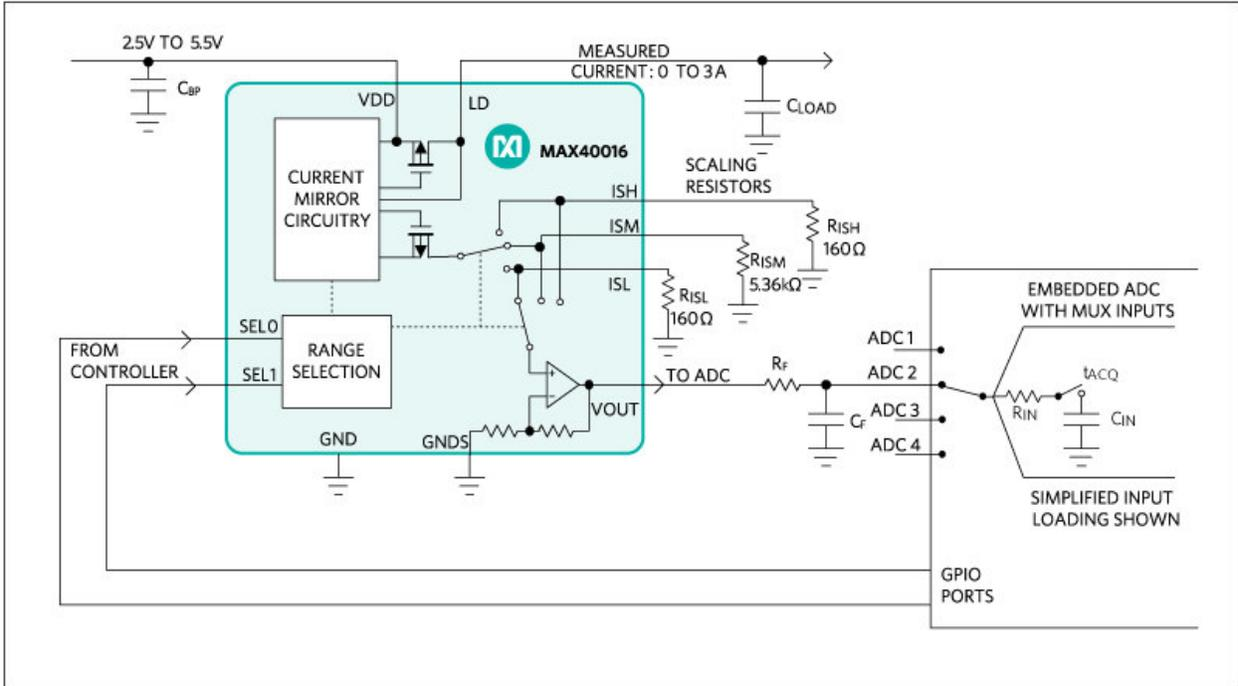
Figure 2. MAX40016 current-sense amplifier is used to measure battery current, while a low-resolution ADC is used to convert output voltage for current monitoring.
