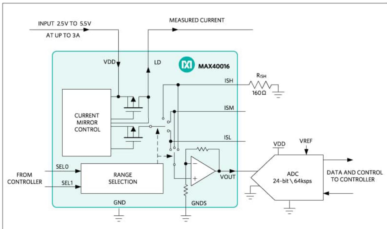
*Figure 1. MAX40016 current-sense amplifier with high-resolution ADC to convert output voltage for current-monitoring.*
