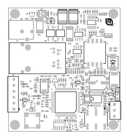
Figure C-2. Component Placement Plot for Bottom
