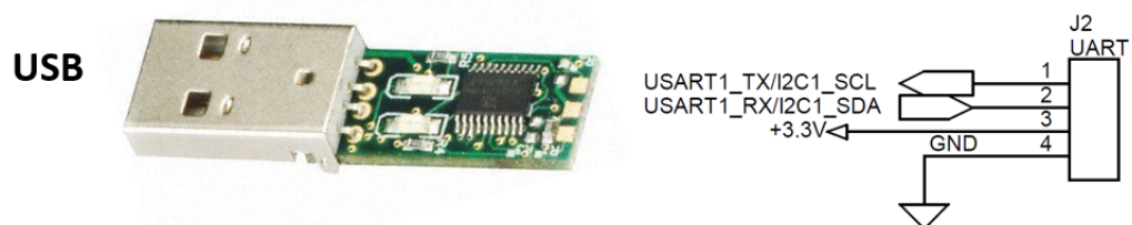
Figure 9. UART TX/RX (3v3 level)
