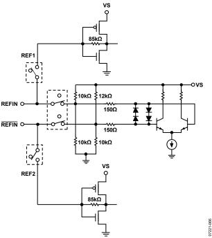
Figure 44. REFIN Equivalent Circuit for NonXTAL Mode
