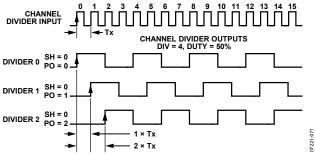
Figure 52. Effect of Coarse Phase Offset (or Delay)
