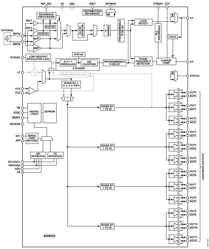
$Figure~38.~High~Frequency~Clock~Distribution \\ -- CLK~or~External~VCO > 1600~MHz~(Mode~2)$
