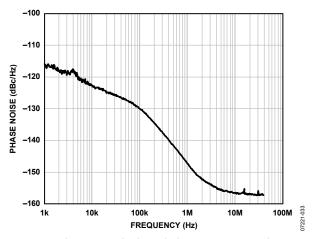
Figure 30. Phase Noise (Absolute) Clock Generation; Internal VCO at 2212 MHz; PFD = 15.36 MHz; LBW = 40 kHz; LVDS Output = 122.88 MHz
