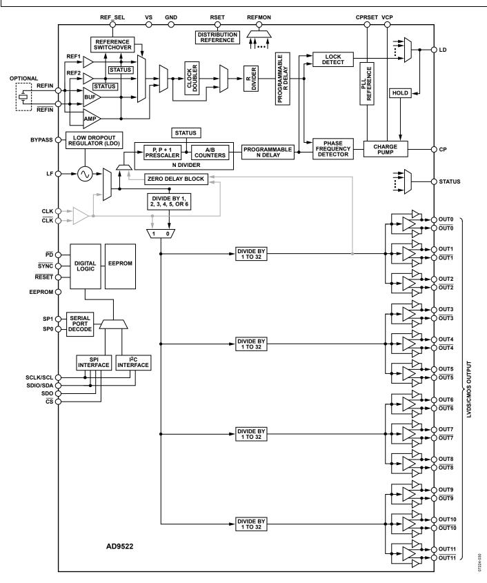
Figure 36. Internal VCO and Clock Distribution (Mode 0)
