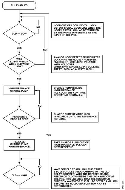
Figure 48. Flowchart of Automatic/Internal Holdover Mode
