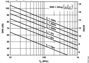
Figure 71. SNR and ENOB vs. Analog Input Frequency
