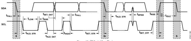
Figure 62. I<sup>2</sup>C Serial Port Timing
