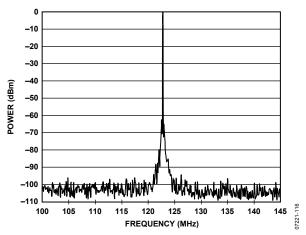
Figure 13. PFD/CP Spurs; 122.88 MHz; PFD = 15.36 MHz; LBW = 127 kHz;  $I_{CP} = 3.0 \text{ mA}$ ;  $f_{VCO} = 2212 \text{ MHz}$
