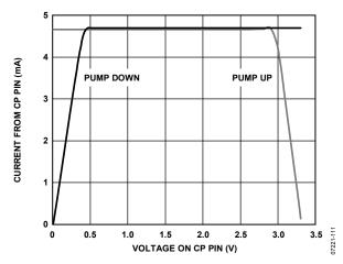
Figure 9. Charge Pump Characteristics at VCP = 3.3 V
