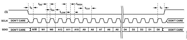
Figure 67. Serial Control Port Read—MSB First, 16-Bit Instruction, Timing Measurements
