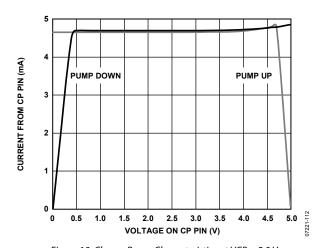
Figure 10. Charge Pump Characteristics at VCP = 5.0 V
