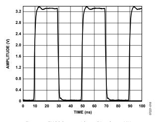
Figure 18. CMOS Output with 10 pF Load at 25 MHz
