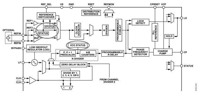
Figure 49. Reference and VCO/CLK Frequency Status Monitors
