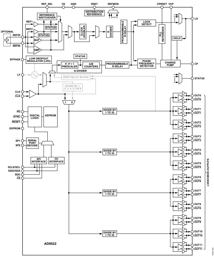
Figure 37. Clock Distribution or External VCO < 1600 MHz (Mode 1)
