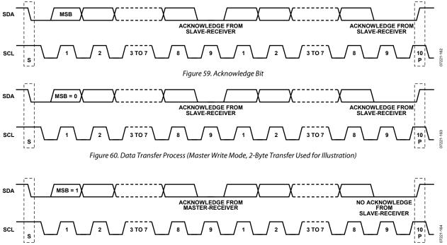
Figure 61. Data Transfer Process (Master Read Mode, 2-Byte Transfer Used for Illustration)
