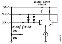
Figure 47. CLK Equivalent Input Circuit
