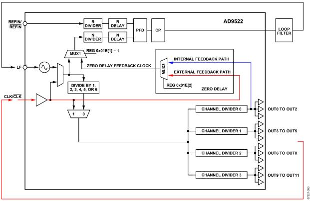
Figure 50. Zero Delay Function
