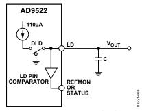
Figure 46. Current Source Digital Lock Detect
