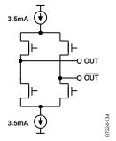
Figure 53. LVDS Output Simplified Equivalent Circuit with 3.5 mA Typical Current Source
