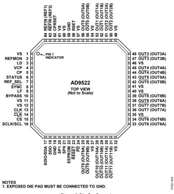
Figure 5. Pin Configuration
