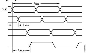
Figure 2.  $CLK/\overline{CLK}$  to Clock Output Timing, DIV = 1
