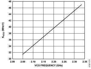
Figure 8. K<sub>VCO</sub> vs. VCO Frequency
