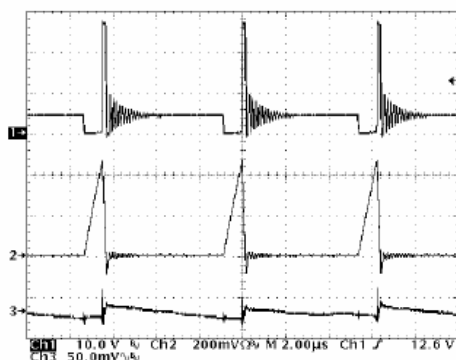
L1 = 8.2 \mu H, C1 = 10 \mu F, C2 = 3.3 \mu F, V_{IN} = 4.2 V, V_{OUT} = 25 V, I_{OUT} = 5.0 mA 1. V_{LX} , 10 V/div 2. I_L , 200 mA/div 3. V_{ripple} , 50 mV/div
