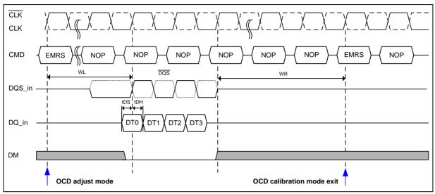
Figure 7 – OCD Adjust Mode
