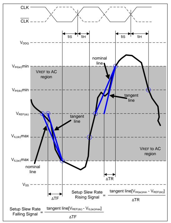
Figure 21 – Illustration of tangent line for tis
