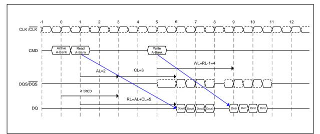
[AL = 2 and CL = 3, RL = (AL + CL) = 5, WL = (RL - 1) = 4, BL = 4]Figure 14 – Example 1: Read followed by a write to the same bank, where AL = 2 and CL = 3, RL = (AL + CL) = 5, WL = (RL - 1) = 4, BL = 4
