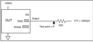
Output slew rate test load
