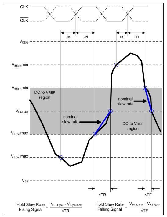
Figure 22 – Illustration of nominal slew rate for till
