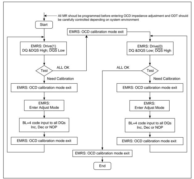
Figure 6 – OCD Impedance Adjustment Flow Chart
