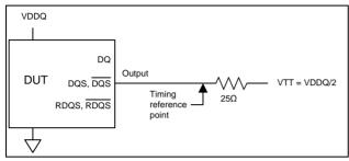
Figure 16 - AC timing reference load
