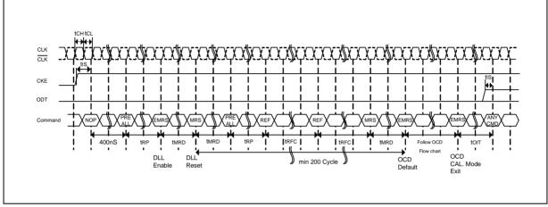
Figure 1 – Initialization sequence after power-up
