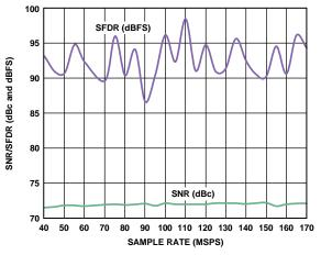
Figure 14. AD9642-170 Single-Tone SNR/SFDR vs. Sample Rate (f<sub>s</sub>) with  $f_{IN} = 90 \, MHz$
