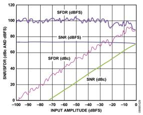
Figure 32. AD9642-250 Single-Tone SNR/SFDR vs. Input Amplitude ( $A_{\rm IN}$ ) with  $f_{\rm IN}=90.1~{\rm MHz}$ ,  $f_{\rm S}=250~{\rm MSPS}$
