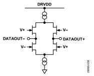
Figure 42. Equivalent LVDS Output Circuit
