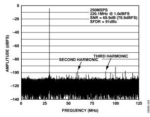
Figure 30. AD9642-250 Single-Tone FFT with  $f_{IN}$  = 220.1 MHz
