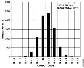
Figure 27. AD9642-210 Grounded Input Histogram,  $f_S = 210$  MSPS
