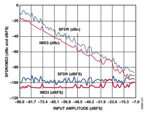
Figure 34. AD9642-250 Two-Tone SFDR/IMD3 vs. Input Amplitude ( $A_{\rm IN}$ ) with  $f_{\rm IN1}=89.12$  MHz,  $f_{\rm IN2}=92.12$  MHz,  $f_{\rm S}=250$  MSPS
