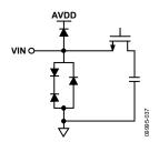
Figure 40. Equivalent Analog Input Circuit
