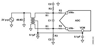
Figure 48. Differential Transformer-Coupled Configuration
