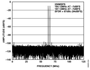
Figure 37. AD9642-250 Two Tone FFT with  $f_{IN1} = 184.12 \text{ MHz}$ ,  $f_{IN2} = 187.12 \text{ MHz}$
