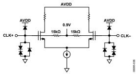
Figure 41. Equivalent Clock Input Circuit
