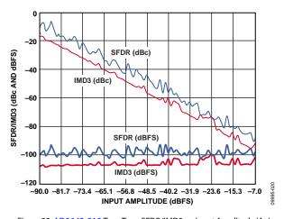
Figure 22. AD9642-210 Two-Tone SFDR/IMD3 vs. Input Amplitude ( $A_{IN}$ ) with  $f_{IN1}=89.12$  MHz,  $f_{IN2}=92.12$  MHz,  $f_{S}=210$  MSPS
