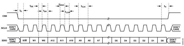
Figure 58. Serial Port Interface Timing Diagram
