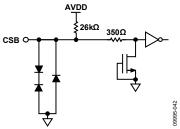
Figure 45. Equivalent CSB Input Circuit
