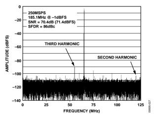
Figure 29. AD9642-250 Single-Tone FFT with  $f_{IN} = 185.1$  MHz
