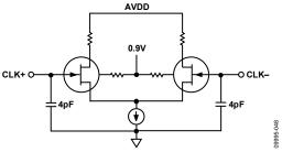
Figure 51. Simplified Equivalent Clock Input Circuit
