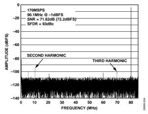
Figure 4. AD9642-170 Single-Tone FFT with  $f_{IN} = 90.1$  MHz
