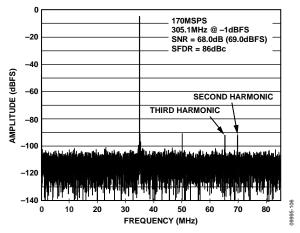
Figure 7. AD9642-170 Single-Tone FFT with  $f_{IN} = 305.1$  MHz
