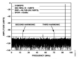
Figure 19. AD9642-210 Single-Tone FFT with  $f_{IN}$  = 305.1 MHz
