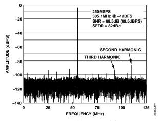
Figure 31. AD9642-250 Single-Tone FFT with  $f_{IN}$  = 305.1 MHz
