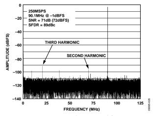
Figure 28. AD9642-250 Single-Tone FFT with  $f_{IN} = 90.1$  MHz
