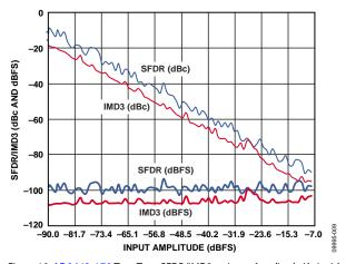
Figure 10. AD9642-170 Two-Tone SFDR/IMD3 vs. Input Amplitude (A<sub>IN</sub>) with  $f_{IN1} = 89.12 \text{ MHz}, f_{IN2} = 92.12 \text{ MHz}, f_S = 170 \text{ MSPS}$
