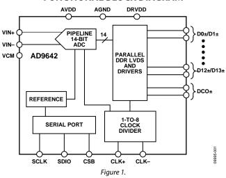
Programming for setup and control is accomplished using a 3-wire SPI-compatible serial interface.
