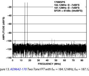
Figure 13. AD9642-170 Two Tone FFT with  $f_{\text{IN1}} = 184.12 \text{ MHz}$ ,  $f_{\text{IN2}} = 187.12 \text{ MHz}$
