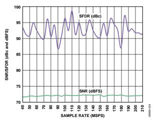
Figure 26. AD9642-210 Single-Tone SNR/SFDR vs. Sample Rate ( $f_s$ ) with  $f_{IN} = 90$  MHz
