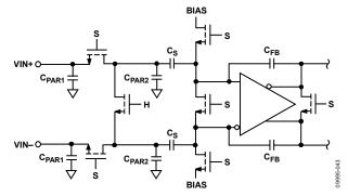
Figure 46. Switched-Capacitor Input
