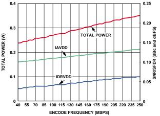
Figure 57. AD9642-250 Power and Current vs. Sample Rate
