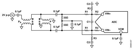
Figure 50. Differential Double Balun Input Configuration
