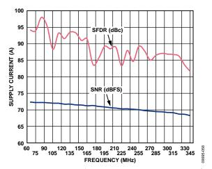
Figure 9. AD9642-170 Single-Tone SNR/SFDR vs. Input Frequency ( $f_{IN}$ ),  $f_{S} = 170$  MSPS
