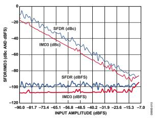
Figure 11. AD9642-170 Two-Tone SFDR/IMD3 vs. Input Amplitude (A<sub>IN</sub>) with  $f_{IN1} = 184.12$  MHz,  $f_{IN2} = 187.12$  MHz,  $f_S = 170$  MSPS
