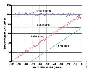
Figure 20. AD9642-210 Single-Tone SNR/SFDR vs. Input Amplitude (A<sub>IN</sub>) with  $f_{\rm IN} = 90.1$  MHz,  $f_{\rm S} = 210$  MSPS
