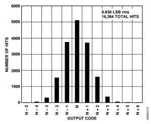
Figure 15. AD9642-170 Grounded Input Histogram,  $f_s = 170 \text{ MSPS}$
