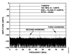
Figure 5. AD9642-170 Single-Tone FFT with  $f_{IN} = 185.1$  MHz
