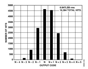
Figure 39. AD9642-250 Grounded Input Histogram,  $f_s = 250 \text{ MSPS}$
