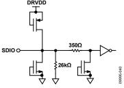
Figure 43. Equivalent SDIO Circuit
