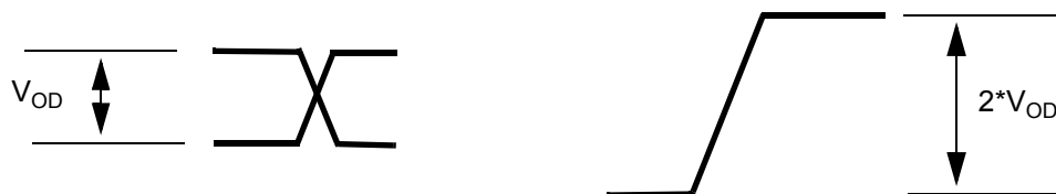
Figure 19 - Differential Output Voltage Parameter
