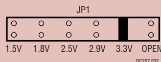
Figure 2. Output Voltage Selection (JP1) (3.3V Position Shown)
