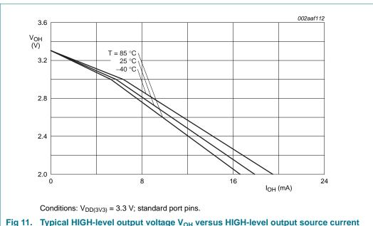
Fig 11. Typical HIGH-level output voltage  $V_{OH}$  versus HIGH-level output source current  $I_{OH}$
