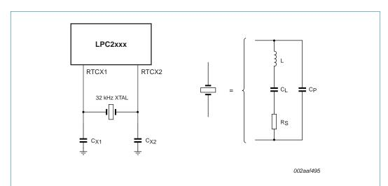
Fig 29. RTC oscillator modes and models: oscillation mode of operation and external crystal model used for  $C_{X1}/C_{X2}$  evaluation
