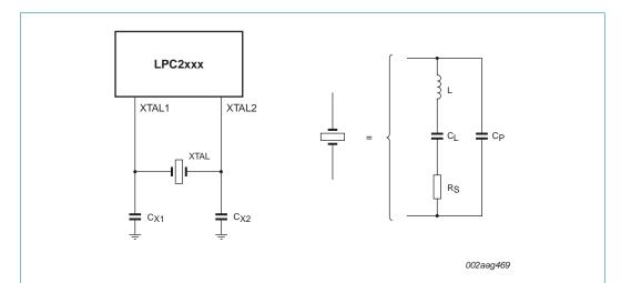
Fig 28. Oscillator modes and models: oscillation mode of operation and external crystal model used for  $C_{X1}/C_{X2}$  evaluation
