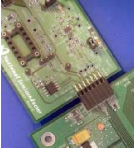
Figure 6: WV4 to ADC121C02XEB Connection
