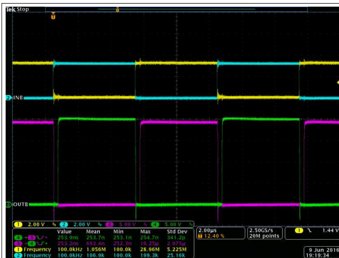
Figure 42. Bench Test Waveform for INA/B and OUTA/B
