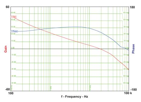
Figure 14. Bottom Converter Loop Response, Vin=36V, Iout=1.0A
