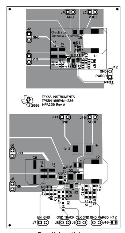
Figure 16. Assembly Layer
