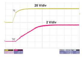
Figure 10. Top Converter Start-up relative to Vin, Vin=42V, lout=1.5A
