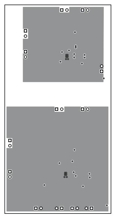
Figure 19. Layer 3 Routing
