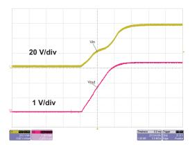
Figure 12. Bottom Converter Start-up relative to Vin, Vin=60.0V, lout=1.5A
