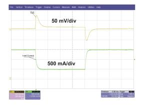
Figure 4. Top Converter Transient Response, 0.5A to 1.5A step, Vin=42V
