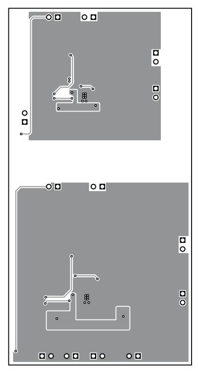
Figure 20. Bottom Layer Routing
