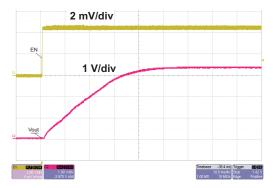
Figure 13. Bottom Converter Start-up relative to EN, Vin=60.0V, lout=1.5A
