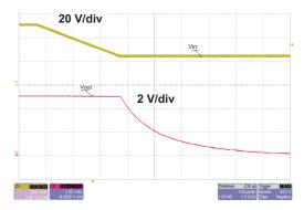
Figure 11. Top Converter UVLO relative to Vin, lout=1.5A
