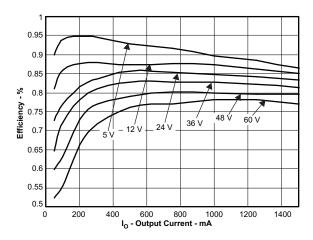
Figure 3. Bottom Converter Efficiency
