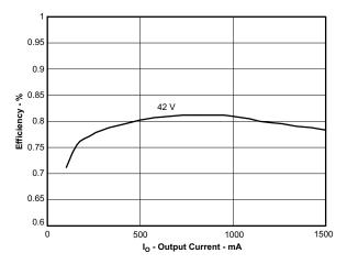
Figure 2. Top Converter Efficiency
