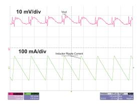
Figure 6. Top Converter Output Voltage Ripple, Vin=42V, lout=1.5A
