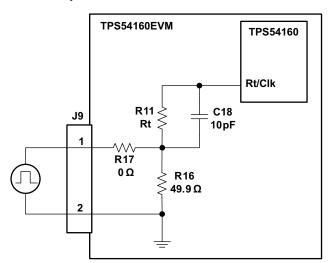
Figure 1. Synchronization to an External Clock
