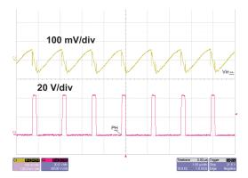
Figure 8. Top Converter Input Voltage Ripple, Vin=42.0V, lout=1.5A
