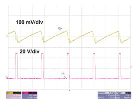
Figure 9. Bottom Converter Input Voltage Ripple, Vin=48.0V, Iout=1.5A
