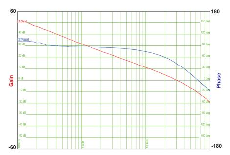
Figure 15. Top Converter Loop Response, Vin=42V, lout=1.0A
