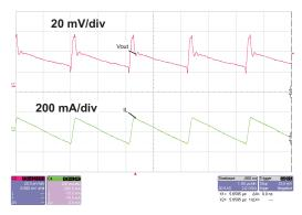
Figure 7. Bottom Converter Output Voltage Ripple, Vin=60.0V, lout=1.5A
