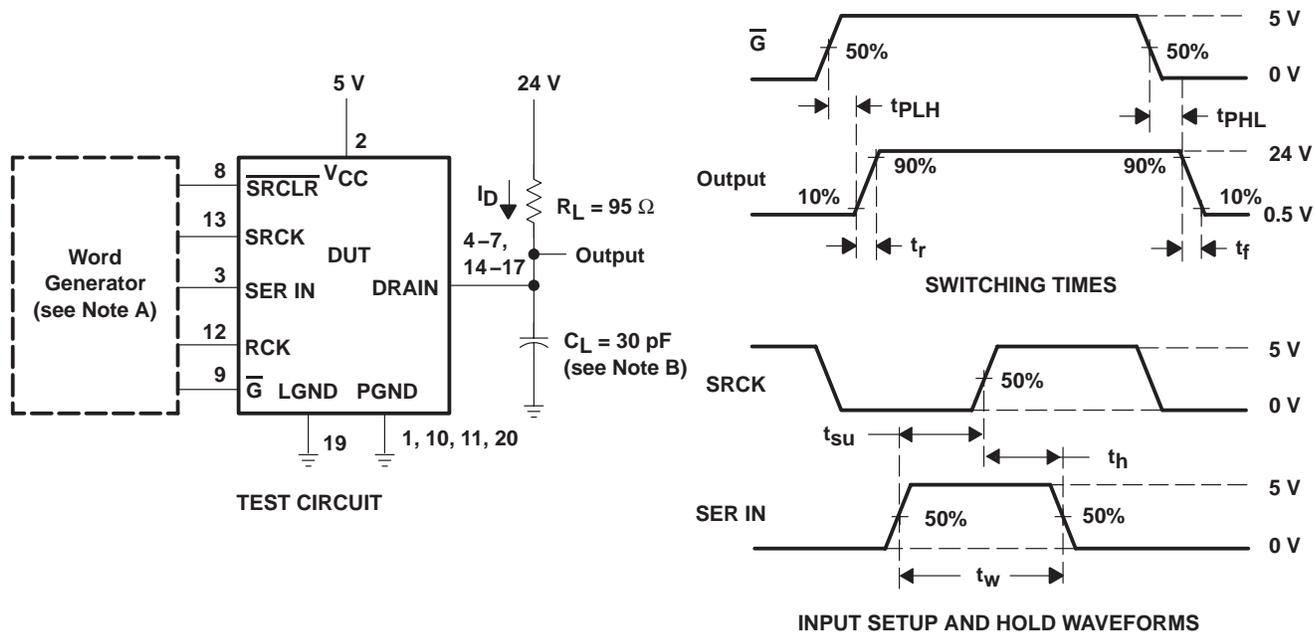
**Figure 2. Test Circuit, Switching Times, and Voltage Waveforms**
