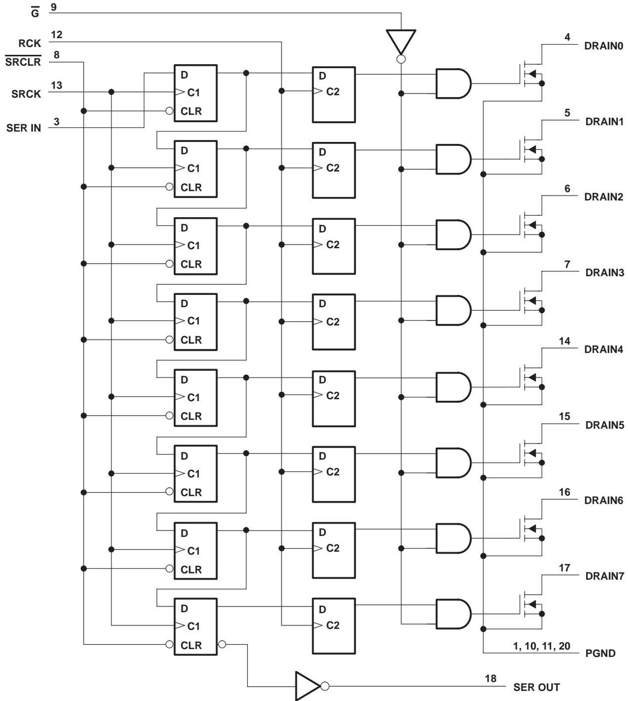
**schematic of inputs and outputs**
