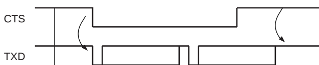
Figure 38-28. Transmitter Behavior when Operating with Hardware Handshaking
