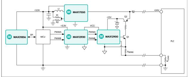
Figure 4. A 3-wire sensor transmitter with DC-DC converter.
