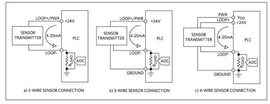
Figure 1. Sensor transmitter connection types.
