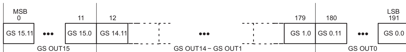
Figure 21. Grayscale Data Packet Format
