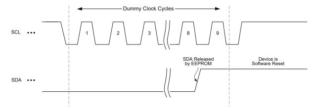
In the event that the device is still non-responsive or remains active on the SDA bus, a power cycle must be used to reset the device (see 4.5.1 Power-Up Requirements and Reset Behavior).
