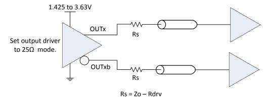
Figure 3.4. LVCMOS Output Termination Example, Option 2
