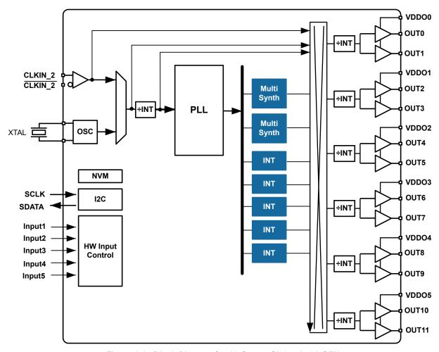
Figure 3.1. Block Diagram for 12-Output Si5357 in 32-QFN
