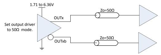
Figure 3.3. LVCMOS Output Termination Example, Option 1
