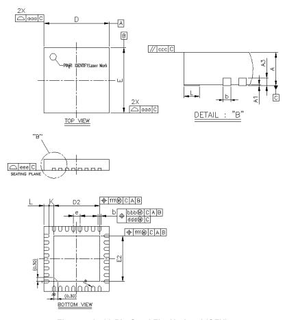
Figure 7.1. 32-Pin Quad Flat No-Lead (QFN)
