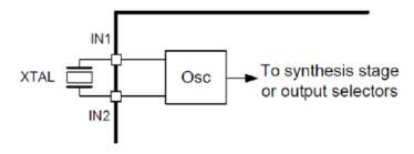
Figure 3.2. External Reference Input (XA/XB)
