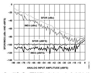
Figure 20. Two Tone SFDR/IMD3 vs. Analog Input Amplitude (A<sub>IN</sub>) with  $f_{\rm IN1}=303.5$  MHz and  $f_{\rm IN2}=306.5$  MHz
