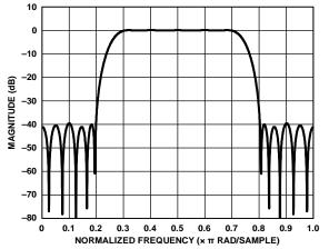
Figure 83. High-Pass, Half-Band Filter Response
