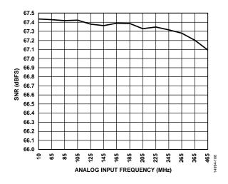
Figure 14. SNR vs. Analog Input Frequency ( $f_N$ ), First and Second Nyquist Zones;  $A_N$  at -3 dBFS
