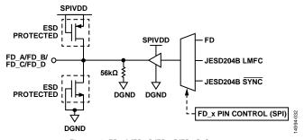
Figure 53. FD\_A/FD\_B/FD\_C/FD\_D Outputs
