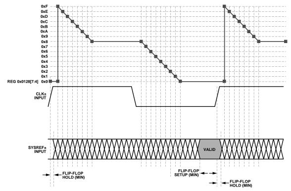
Figure 104. SYSREF± Hold Detector
