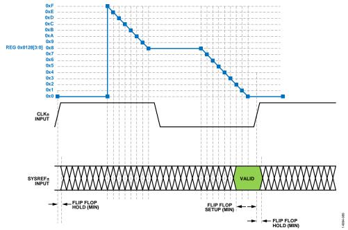
Figure 103. SYSREF± Setup Detector
