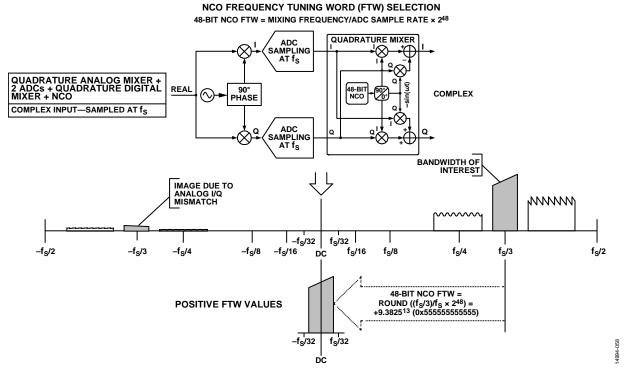
Figure 76. DDC NCO Frequency Tuning Word Selection—Complex Inputs
