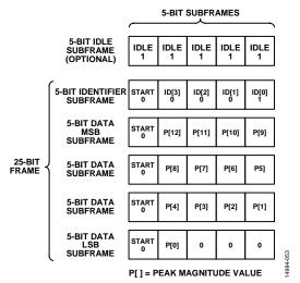
Figure 71. SPORT over JESD204B Signal Monitor Frame Data
