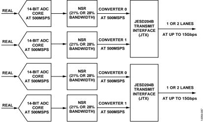
Figure 101. Two ADC + NSR Mode
