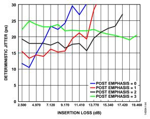
Figure 94. Deterministic Jitter vs. Insertion Loss
