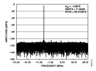
Figure 31. DDC Mode (4 DDCs, Decimate by 8, L, M, and F = 148) with  $f_{\rm IN} = 305~{\rm MHz}$
