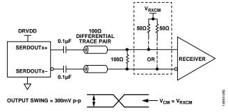
Figure 92. AC-Coupled Digital Output Termination Example
