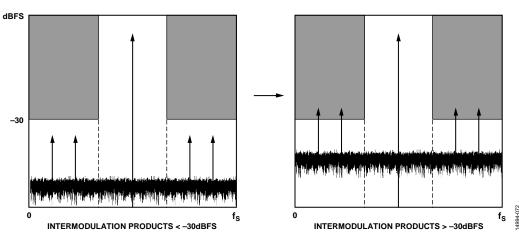
Figure 84. VDR Operation—Reduction in Output Resolution
