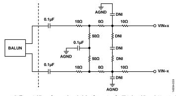
Figure~58.~Differential~Transformer~Coupled~Configuration~for~Third~and~Fourth~Nyquist~Zones~Aller for~Third~and~Fourth~Nyquist~Zones~Aller for~Third~and~Aller for~Third~a
