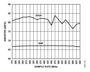
Figure 12. SNR/SFDR vs. Sample Rate ( $f_s$ ),  $f_{IN} = 155$  MHz
