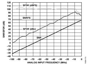
Figure 21. SNR/SFDR vs. Analog Input Frequency,  $f_{IN} = 155$  MHz
