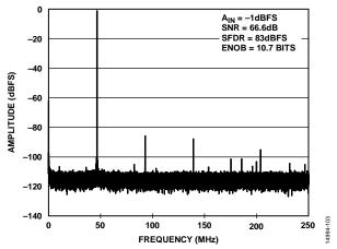
Figure 9. Single-Tone FFT with  $f_{IN} = 453 \text{ MHz}$
