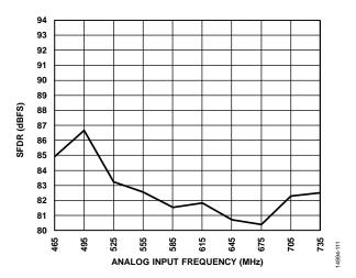
Figure 17. SFDR vs. Analog Input Frequency ( $f_{\rm IN}$ ), Third Nyquist Zone;  $A_{\rm IN}$  at -3 dBFS
