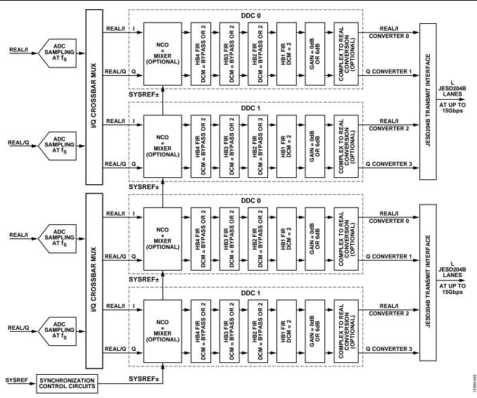
Figure 73. DDC Detailed Block Diagram
