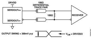
Figure 93. DC-Coupled Digital Output Termination Example
