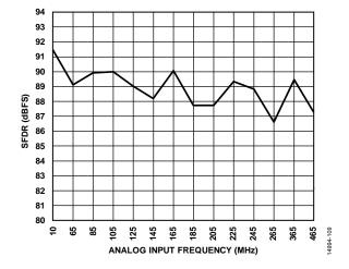
Figure 15. SFDR vs. Analog Input Frequency ( $f_{\rm IN}$ ), First and Second Nyquist Zones;  $A_{\rm IN}$  at -3 dBFS
