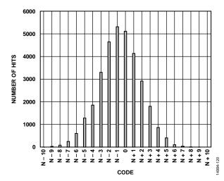
Figure 26. Input-Referred Noise Histogram
