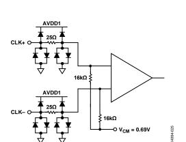
Figure 46. Clock Inputs
