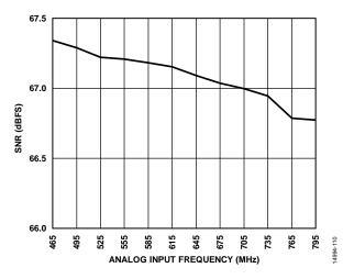
Figure 16. SNR vs. Analog Input Frequency ( $f_{\rm IN}$ ), Third Nyquist Zone  $A_{\rm IN}$  at -3 dBFS
