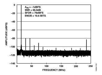
Figure 11. Single-Tone FFT with  $f_{IN} = 985 \text{ MHz}$
