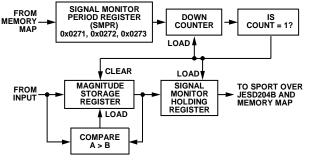
Figure 69. Signal Monitor Block
