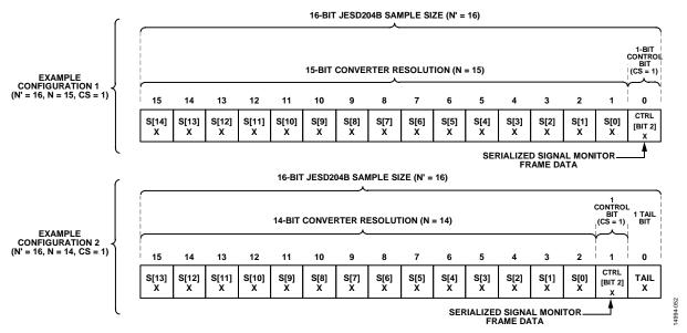
Figure 70. Signal Monitor Control Bit Locations
