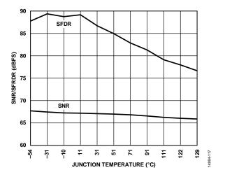
Figure 23. SNR/SFDR vs. Junction Temperature,  $f_{\text{IN}} = 155 \text{ MHz}$
