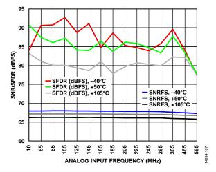
Figure 13. SNR/SFDR vs. Analog Input Frequency (f<sub>IN</sub>)
