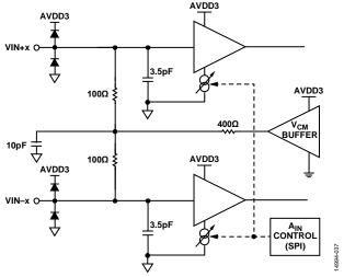
Using Register 0x1A4C and Register 0x1A4D, the buffer currents on each channel can be scaled to optimize the SFDR over various input frequencies and bandwidths of interest. As the input buffer currents are set, the amount of current required by the AVDD3 supply changes. This relationship is shown in Figure 59. For a complete list of buffer current settings, see Table 46.
