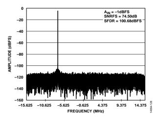
Figure 32. DDC Mode (4 DDCs, Decimate by 16, L, M, and F = 148) with  $f_{\rm IN}$  = 305 MHz
