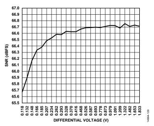
Figure 35. SNR vs. Clock Amplitude (Differential Voltage),  $f_{IN} = 155.3 \text{ MHz}$
