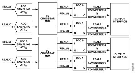
Figure 99. DDCs and Virtual Converter Mapping
