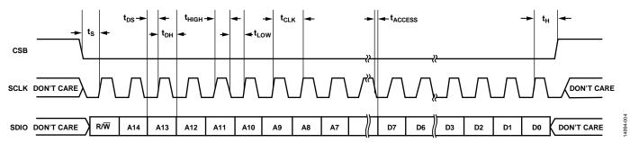
Figure 4. Serial Port Interface Timing Diagram
