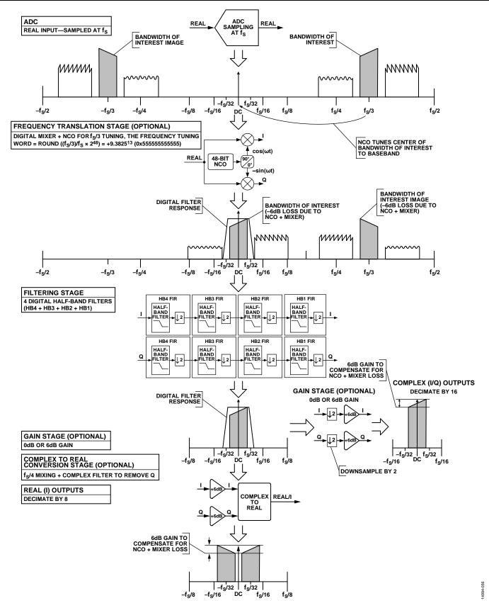
Figure 74. DDC Theory of Operation Example (Real Input, Decimate by 16)
