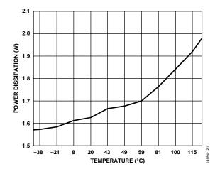
Figure 27. NSR Mode Power Dissipation vs. Junction Temperature
