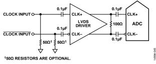
Figure 64. Differential LVDS Sample Clock
