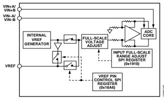
Figure 60. Internal Reference Configuration and Controls
