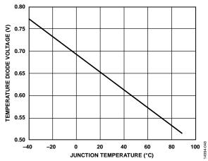
Figure 67. Temperature Diode Voltage vs. Junction Temperature
