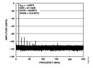
Figure 6. Single-Tone FFT with  $f_{IN} = 10.3 MHz$
