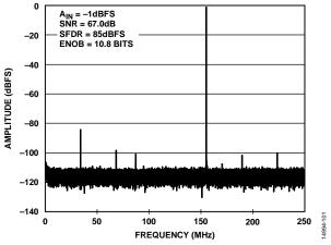
Figure 7. Single-Tone FFT with  $f_{IN} = 155 \text{ MHz}$
