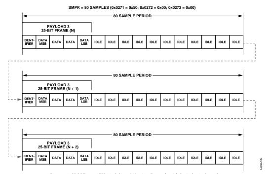
Figure 72. SPORT over JESD204B Signal Monitor Example with Period = 80 Samples
