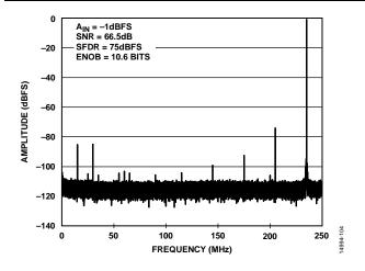
Figure 10. Single-Tone FFT with  $f_{IN} = 765 \text{ MHz}$
