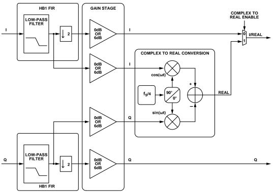
Figure 81. Complex to Real Conversion Block
