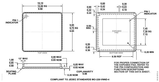
Figure 107. 72-Lead Lead Frame Chip Scale Package [LFCSP] 10 mm × 10 mm Body and 0.85 mm Package Height (CP-72-10) Dimensions shown in millimeters
