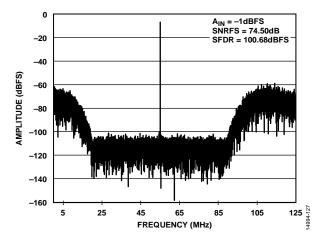
Figure 33. NSR Mode (Decimate by 2, L, M, and F = 124) with  $f_{\rm IN}$  = 305 MHz
