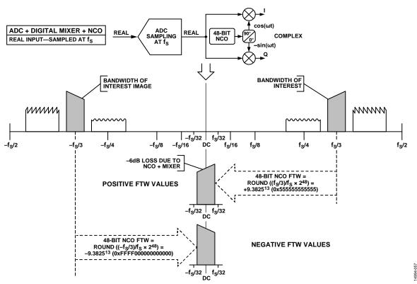
Figure 75. DDC NCO Frequency Tuning Word Selection—Real Inputs
