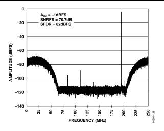
Figure 34. NSR Mode (LMF = 222) with  $f_{IN}$  = 305 MHz
