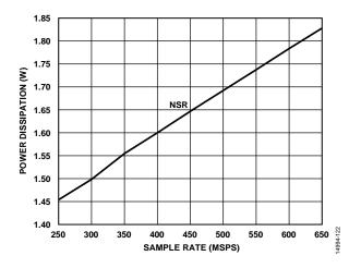
Figure 28. Power Dissipation vs. Sample Rate (fs)
