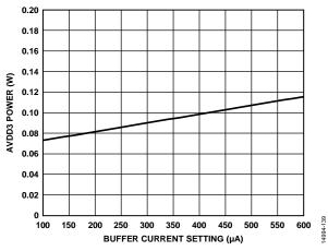
Figure 59. AVDD3 Power vs. Buffer Current Setting
