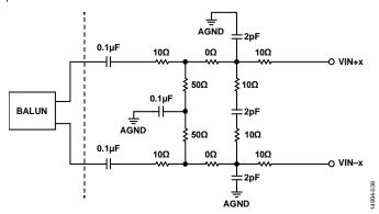
Figure 57. Differential Transformer Coupled Configuration for First and Second Nyquist Frequencies
