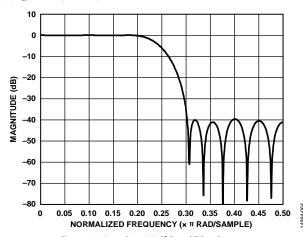
Figure 82. Low-Pass, Half-Band Filter Response
