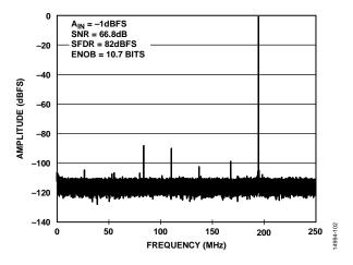
Figure 8. Single-Tone FFT with  $f_{IN} = 305 \text{ MHz}$
