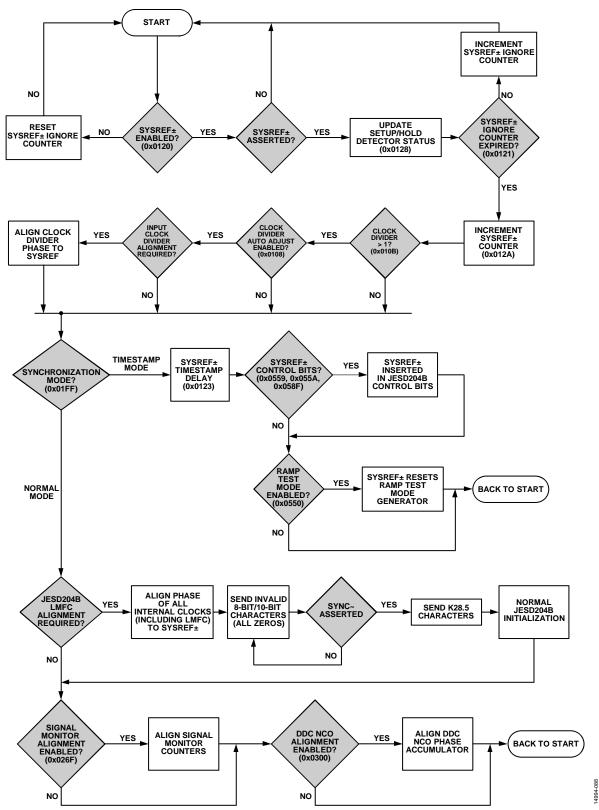
Figure 102. Multichip Synchronization
