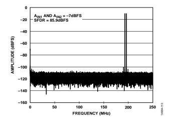
Figure 19. Two Tone FFT;  $f_{IN1} = 303.5 \text{ MHz}$ ,  $f_{IN2} = 306.5 \text{ MHz}$
