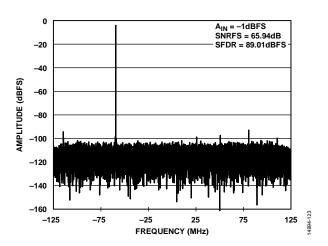
Figure 29. DDC Mode (4 DDCs, DCM2, L, M, and F = 244) with  $f_{\mathbb{N}}$  = 305 MHz
