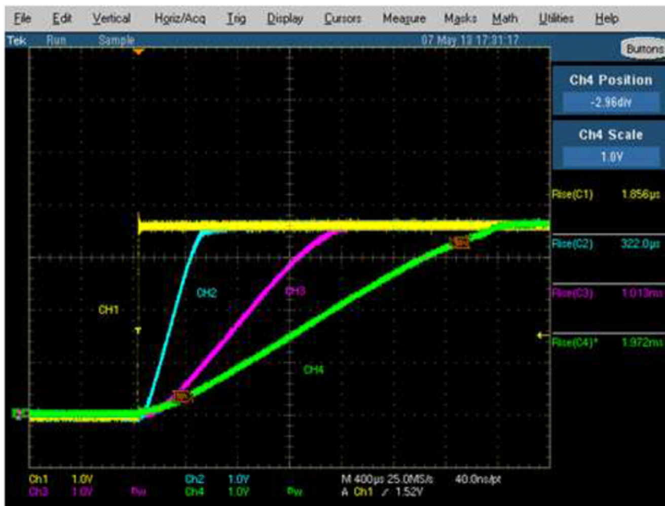
Figure 32. Programmable Slew Rate Control
