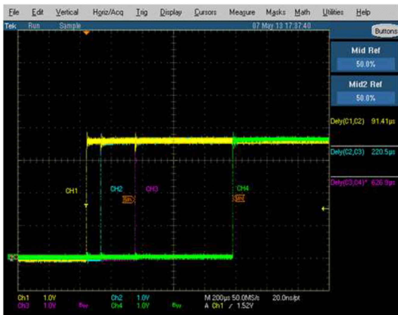
Figure 33. Programmable Turn on Delay Time
