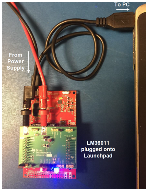
Figure 6. LM36011EVM Test Setup
