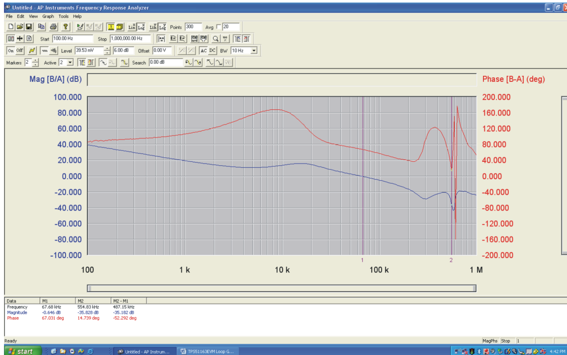
Figure 7. Loop Response Gain and Phase
