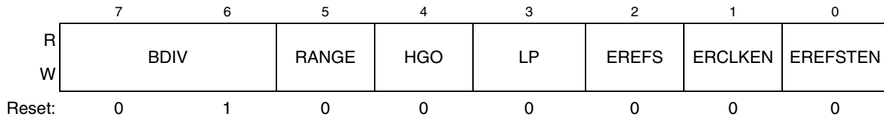
Figure 8-4. ICS Control Register 2 (ICSC2)
